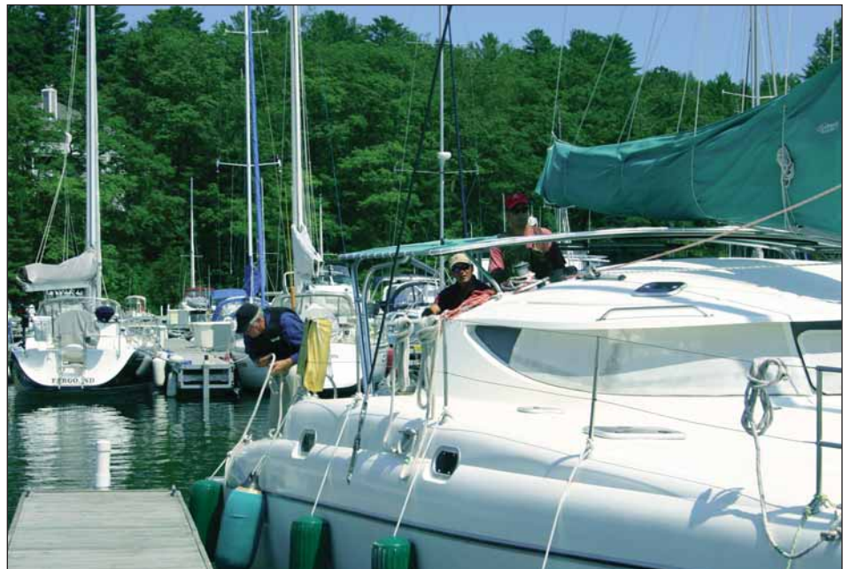
With the bow sprung out against the wind the stern line is cast off.
