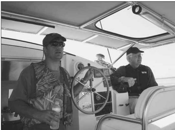
Dave drives Calico backwards using the engines to steer while Ed assists by holding the wheel centered.
