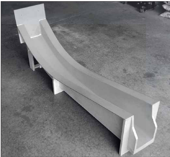
Completed beam mold for Scarab 650.
