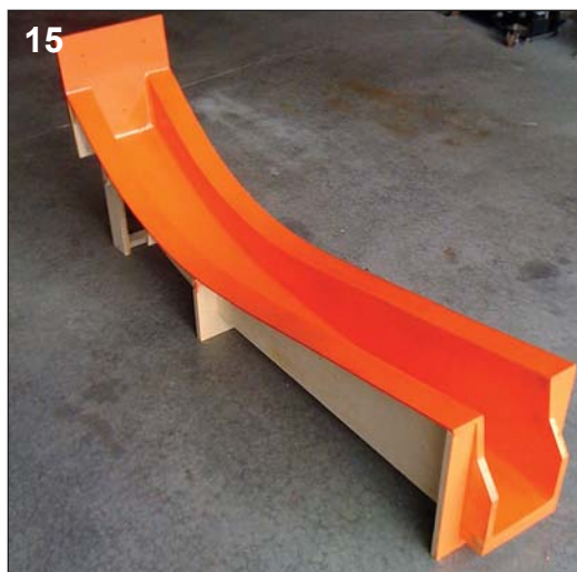
Page 15, Completed Beam mold for Scarab 650 Trimaran. Photo by Rich Kurlinski
