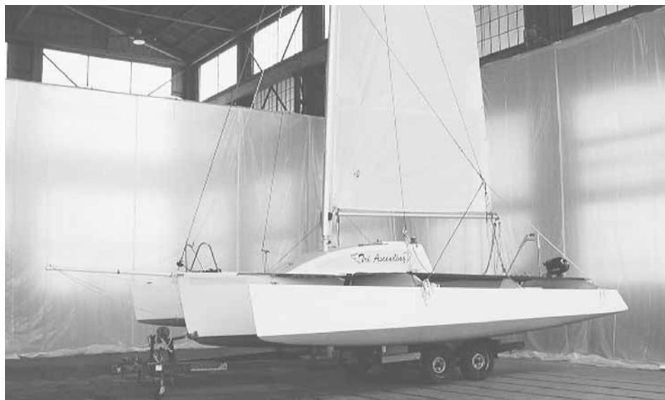
Figure 5 - A completed L7 trimaran. When folded, the L-7 is 8'4" wide and easily trailered.
