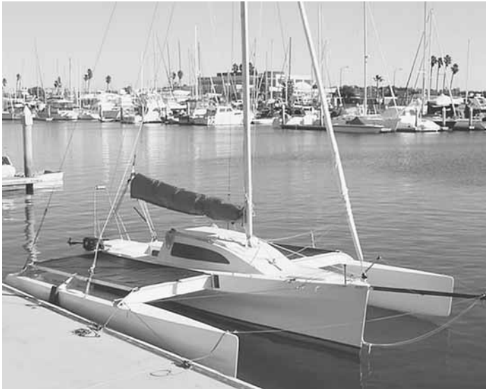
Figure 1 - A completed L-7 at the dock, Multi Marine's new 23' folding trimaran kit features manufactured hull pans. The builder attaches plywood topsides to the pans.
